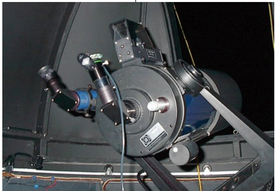
My setup. I placed the circuit board of the webcam in the end of a film canister so it would fit in my eyepiece holder.
